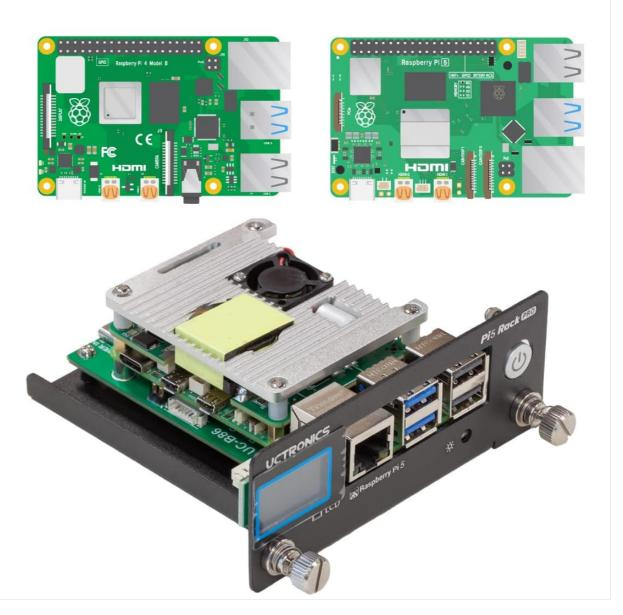
This image illustrates the compatibility of the PoE Hat with Raspberry Pi 3B+, 4B, and 5 models. It also shows the PoE Hat installed on a Raspberry Pi within a UCTRONICS rackmount, demonstrating its compact integration.
