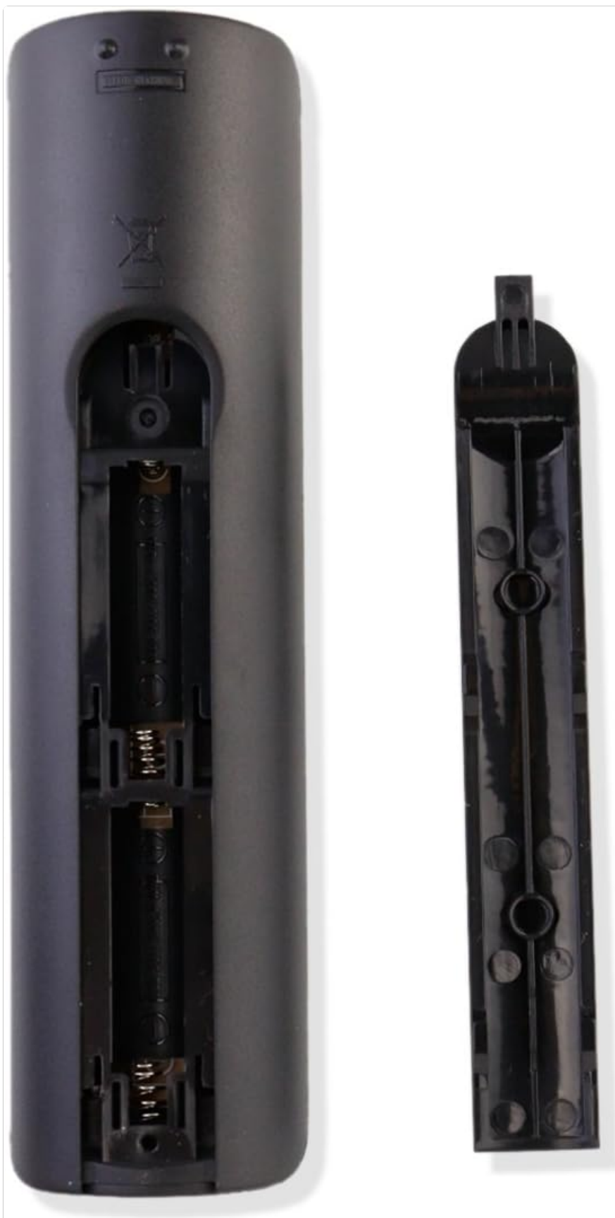
Figure 1: Back of the remote control with the battery compartment open, illustrating where to insert AAA batteries.
