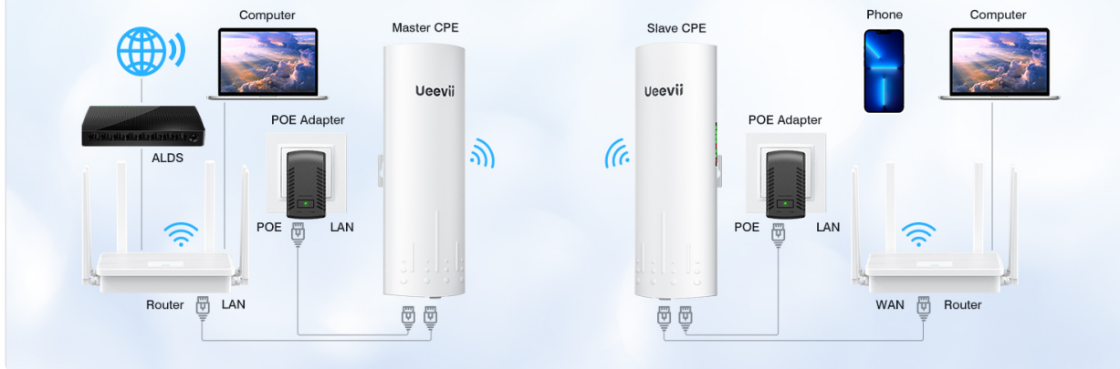
Image: A diagram illustrating the setup for connecting the UeeVii WR3000K router with a wireless bridge (Master CPE and Slave CPE) to extend network coverage.
