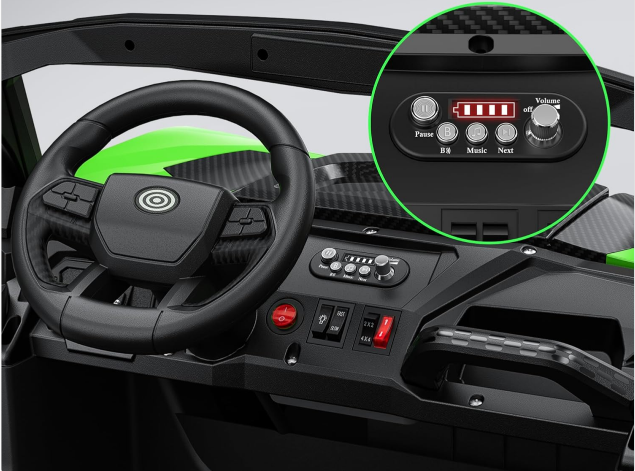
Image: A detailed view of the ride-on car's multifunction dashboard, showing controls for music, lights, volume, and a battery level indicator.
