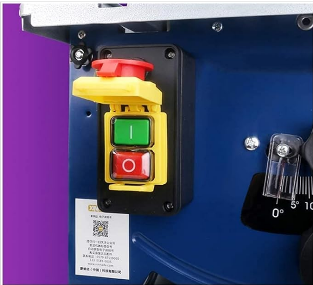
Electromagnetic switch Overload protection function
