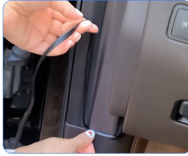
STEP2: The wire is stuffed into the A-pillar seal
