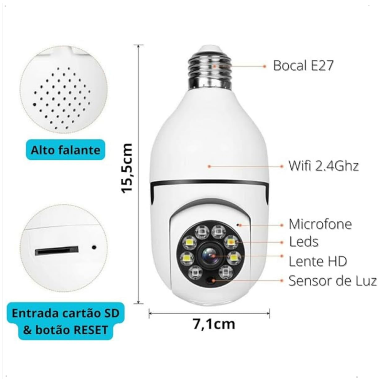
Image 1: Genérico 8177 IP Camera Components and Dimensions. This diagram highlights key features such as the E27 bulb socket for power, the integrated speaker and microphone for two-way audio, HD lens, LED lights for night vision, a light sensor, and the location of the SD card slot and reset button. Dimensions are also indicated.
