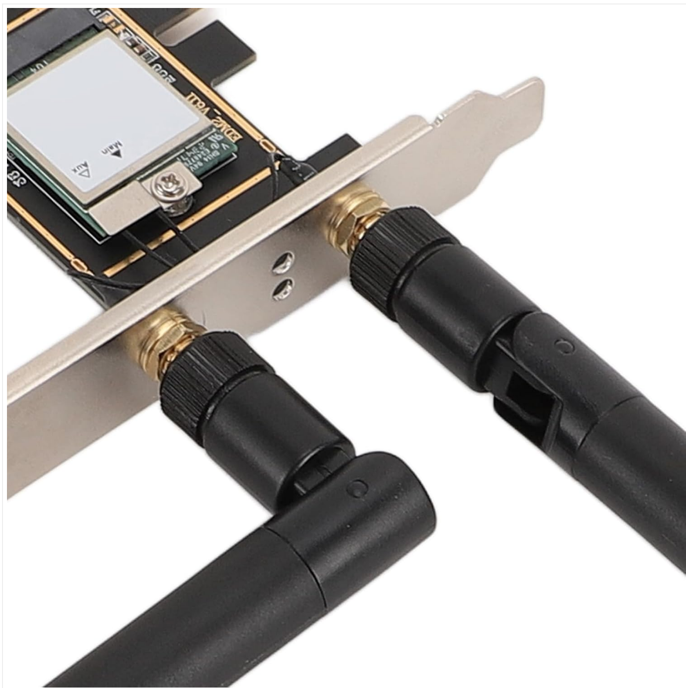
Figure 4: Detail of antenna connection points.
