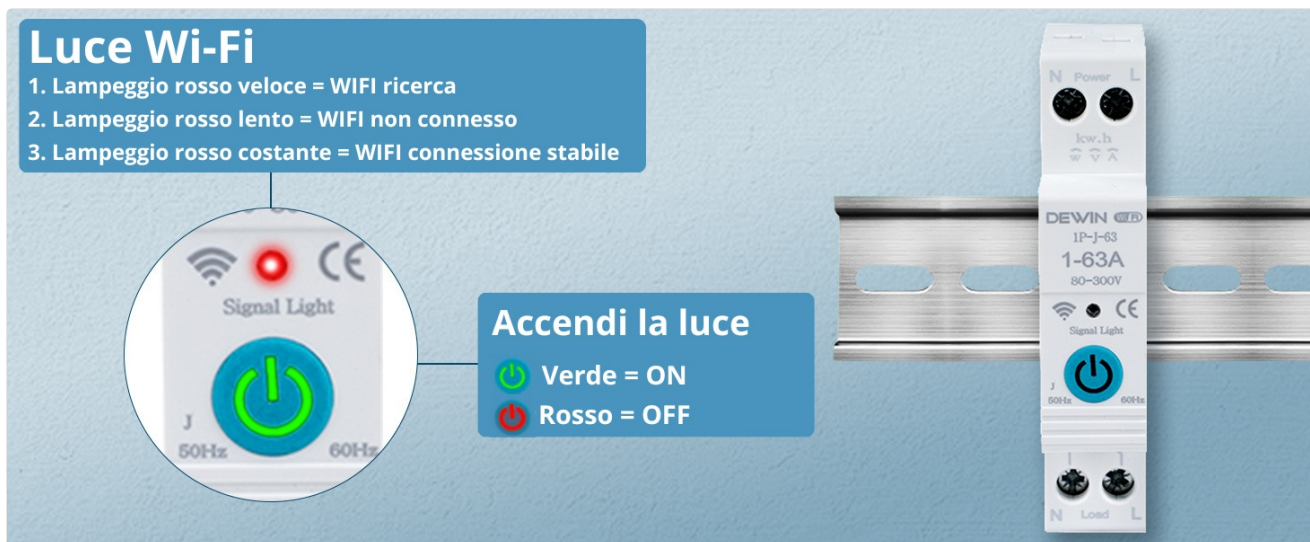
Figure 4: WiFi and Power Indicator Lights. This image details the meaning of the WiFi signal light's different flashing patterns and the power button's color (Green for ON, Red for OFF).
