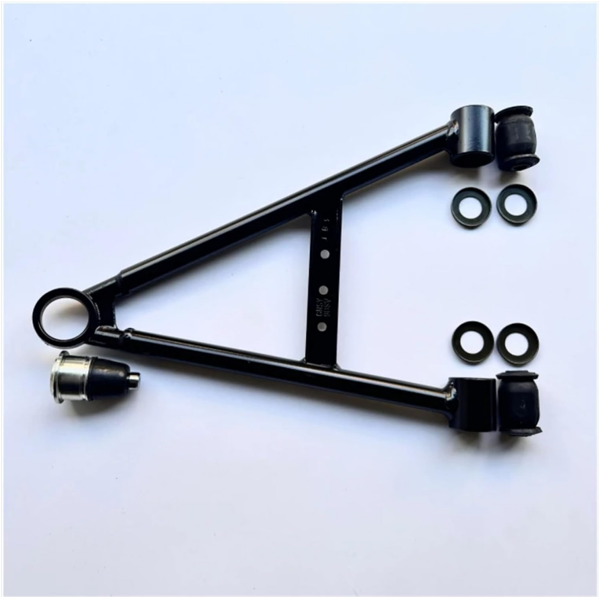
Figure 5.1: View of the swing arm's mounting points and ball joint.
