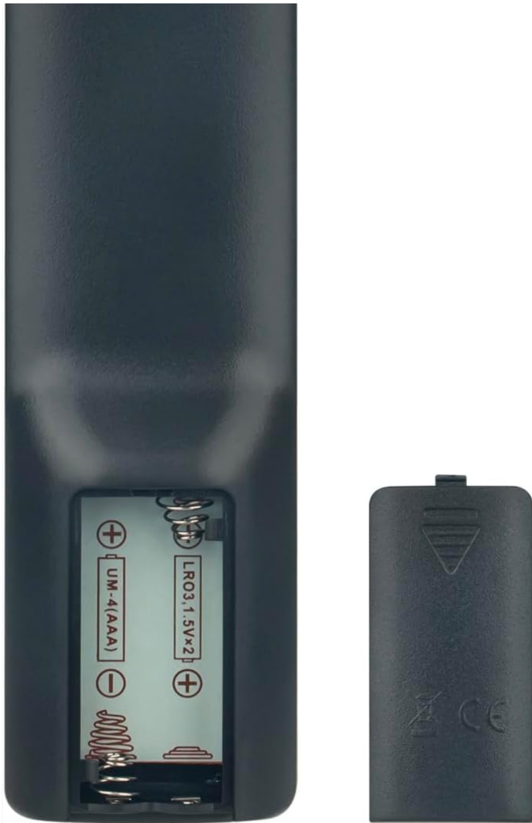
Image 3.1: Back view of the remote control with the battery compartment open, showing where to insert AAA batteries.
