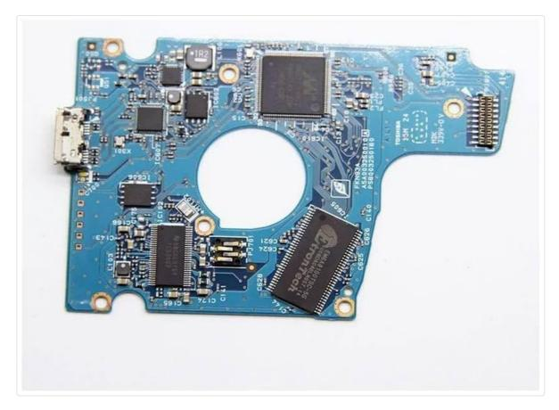
This image displays the top side of the G003250A PCB board, highlighting the main controller chip, USB 3.0 port, and various surface-mounted components. This is the side that interfaces with the hard drive's internal components and provides the external USB connection.
