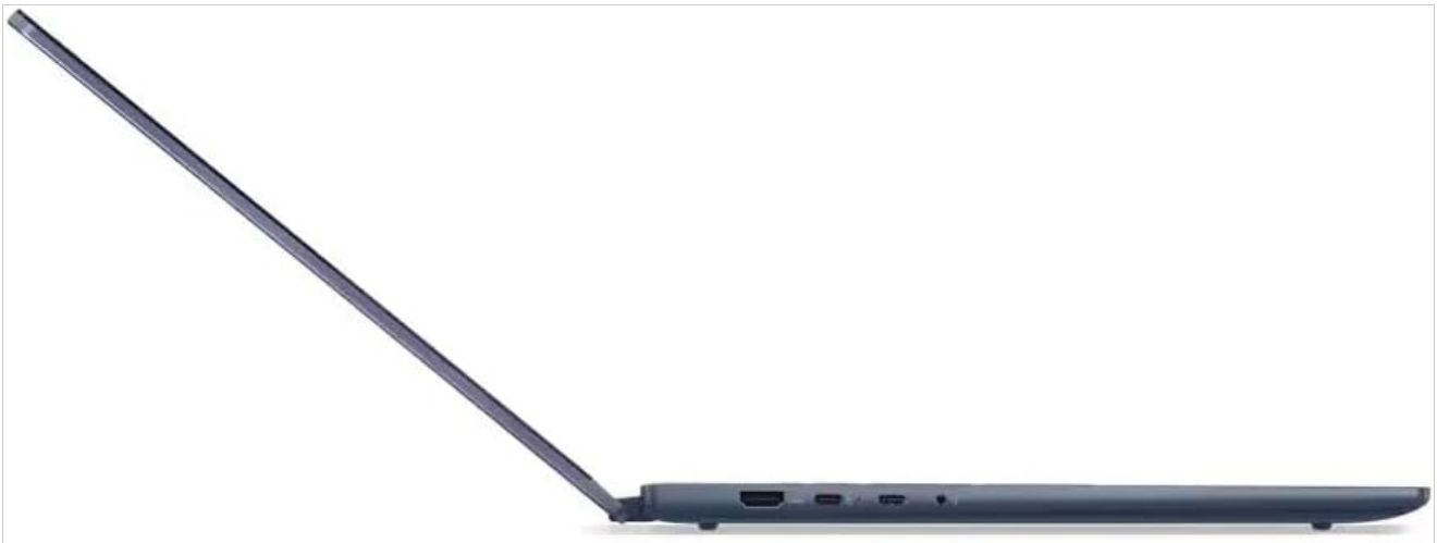
Figure 3.3: Left side ports including USB 3.2 Gen 2 Type-C (Power Delivery/DisplayPort), HDMI v1.4, and Headphone/Microphone Combo Jack.
