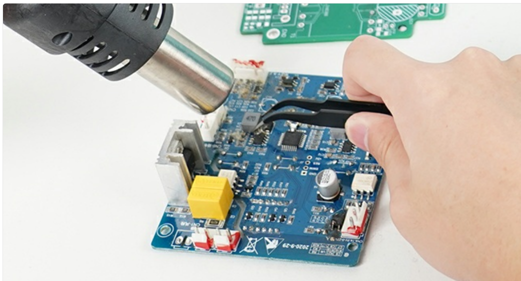
Figure 8: Example of using the hot air gun for electronic rework.
