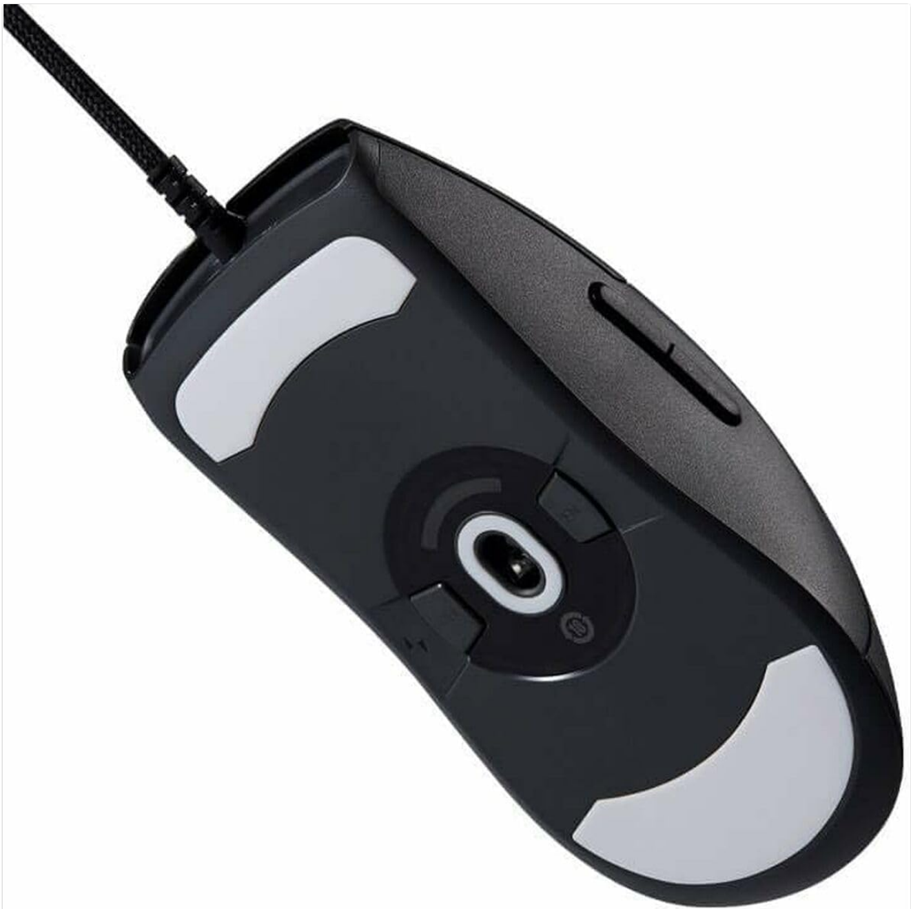
Figure 2.4: Bottom view of the Xiaomi Gaming Mouse Lite, showing the sensor and glide feet.
