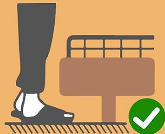
Figure 3: Illustration of the innovative hidden support legs design, allowing for easy cleaning underneath.
