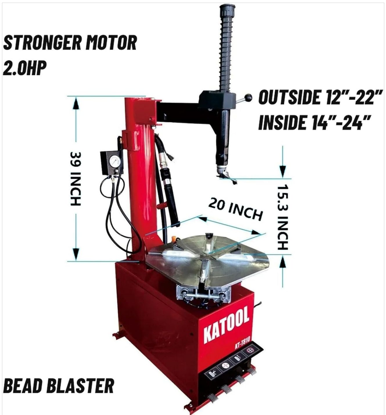
Image: KATOOL KT-T810 Tire Changer, illustrating the side-mounted bead breaker and overall dimensions.
