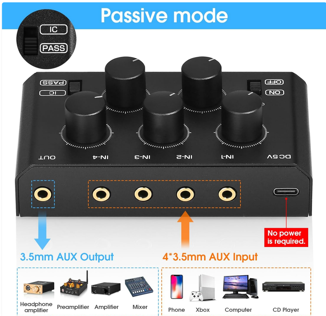
Image 5.1: Connection diagram for the MC5-BX in passive mode, showing inputs from various devices and output to an amplifier.
