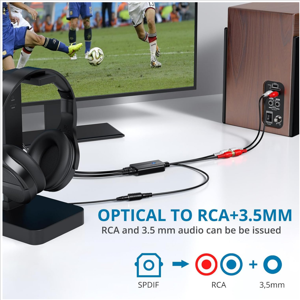
Image: A visual representation illustrating the conversion process from a single SPDIF digital audio input to dual analog outputs: RCA (red and white) and a 3.5mm stereo jack.
