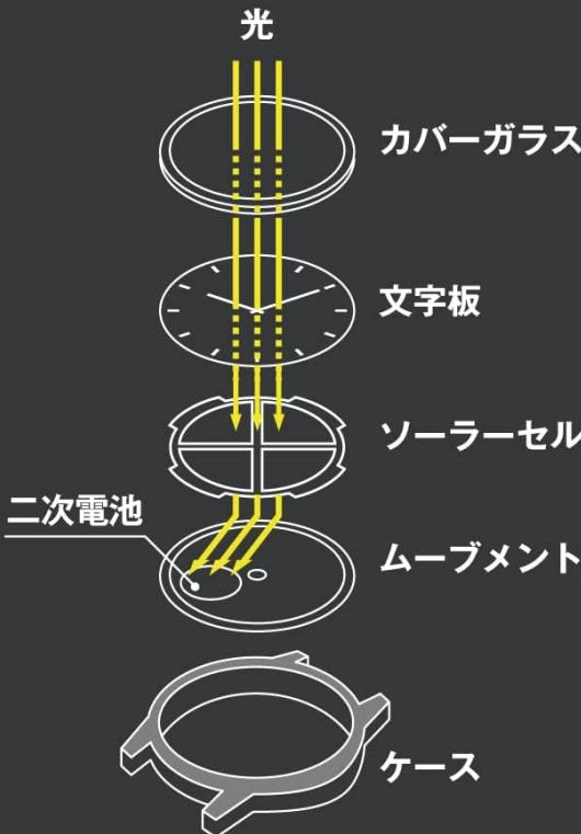
This diagram visually explains how the Eco-Drive system works, showing light passing through the cover glass and dial to reach the solar cell, which converts it into energy stored in a secondary battery to power the movement.
