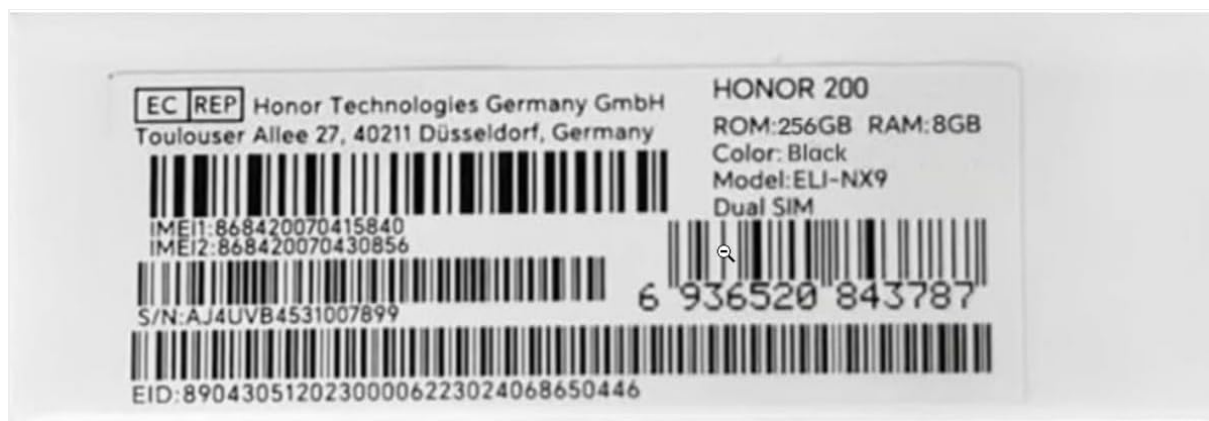
Figure 8.1: Example product label showing model (ELI-NX9), ROM/RAM, color, IMEI, and UPC. This information is unique to each device.
