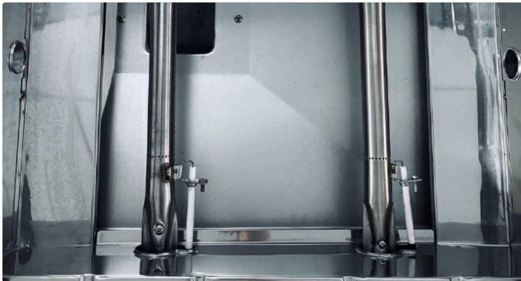
Image: Close-up of the new igniter electrodes and their wiring, ready for installation into the grill's ignition system.
