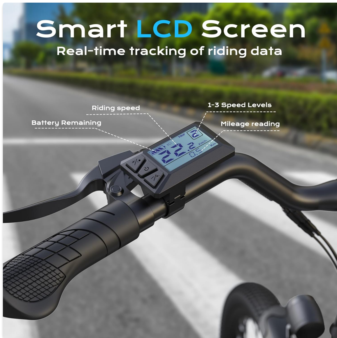
Figure 6: The Smart LCD Screen displaying real-time riding data such as battery remaining, riding speed, 1-3 speed levels, and mileage reading.
