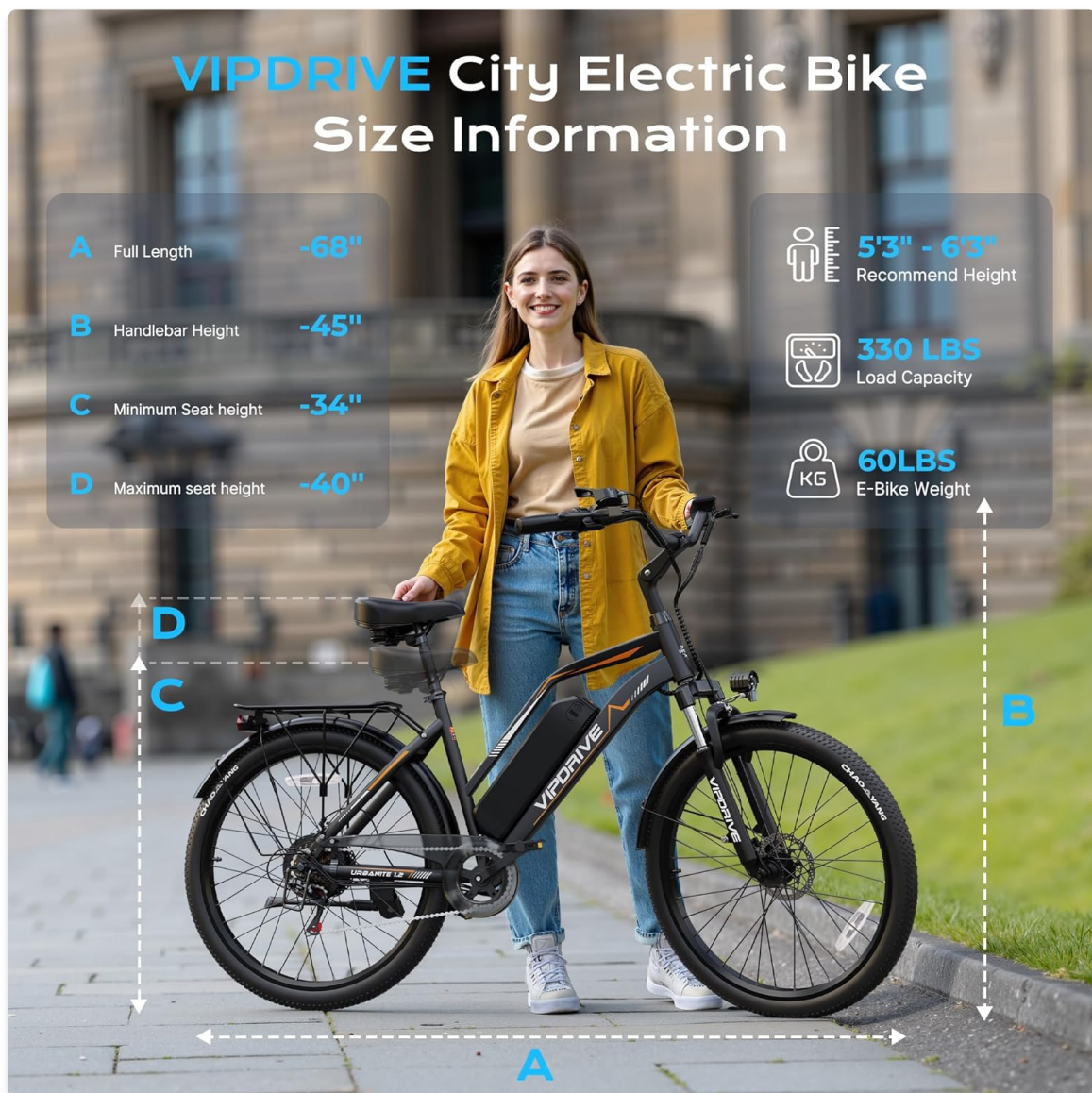
Figure 2: Size information for the Vipdrive Urbanite 1.2 Electric Bike, including full length, handlebar height, minimum seat height, maximum seat height, load capacity, and E-Bike weight.
