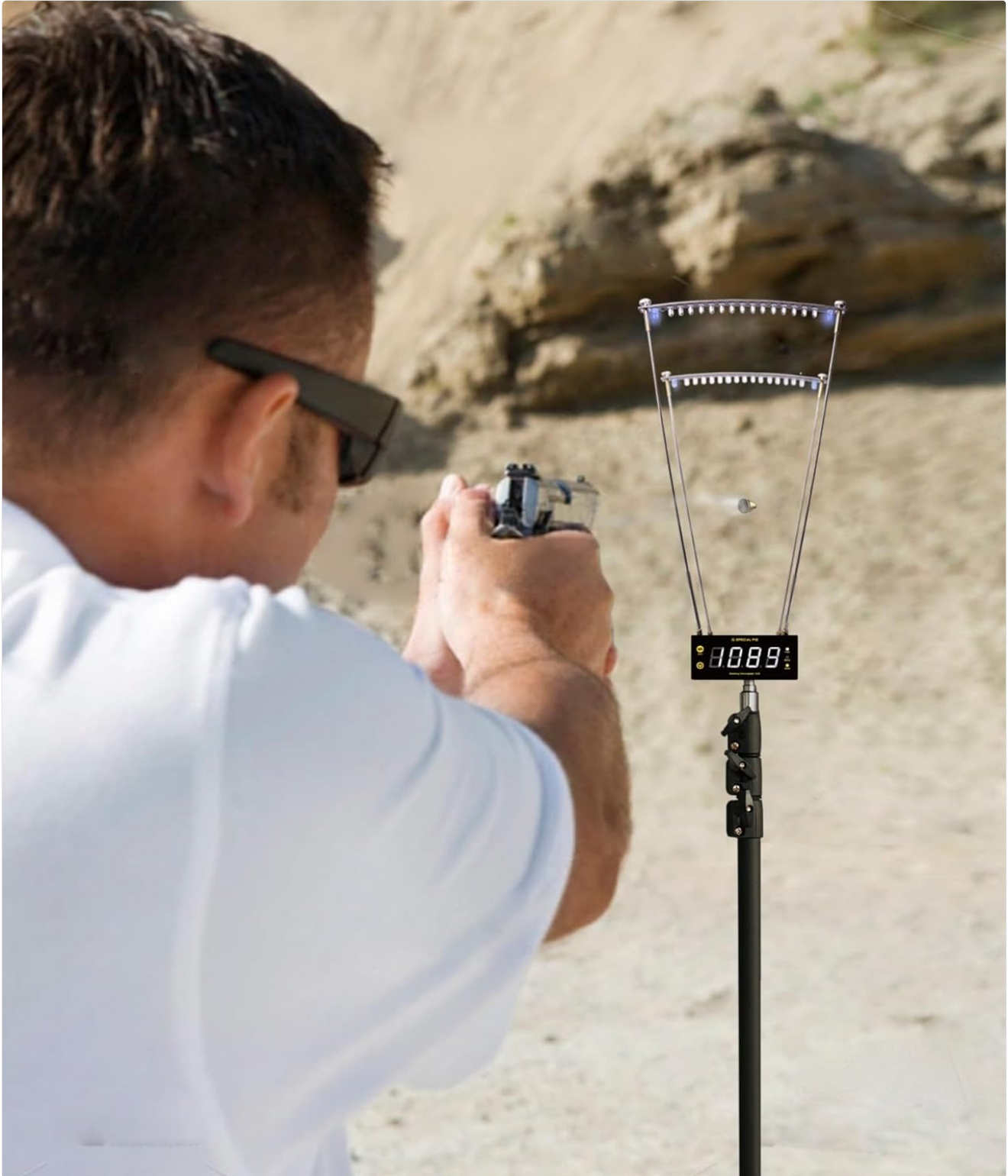
Figure 4.1: Example of using the SC9 Chronograph for velocity measurement.
