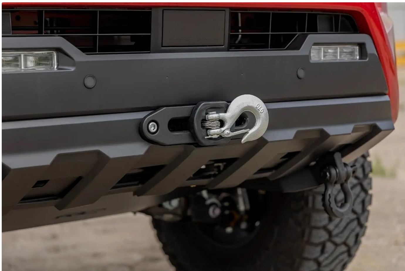
Figure 6: Another perspective of the hawse fairlead and clevis hook, highlighting the robust connection point for recovery operations.
