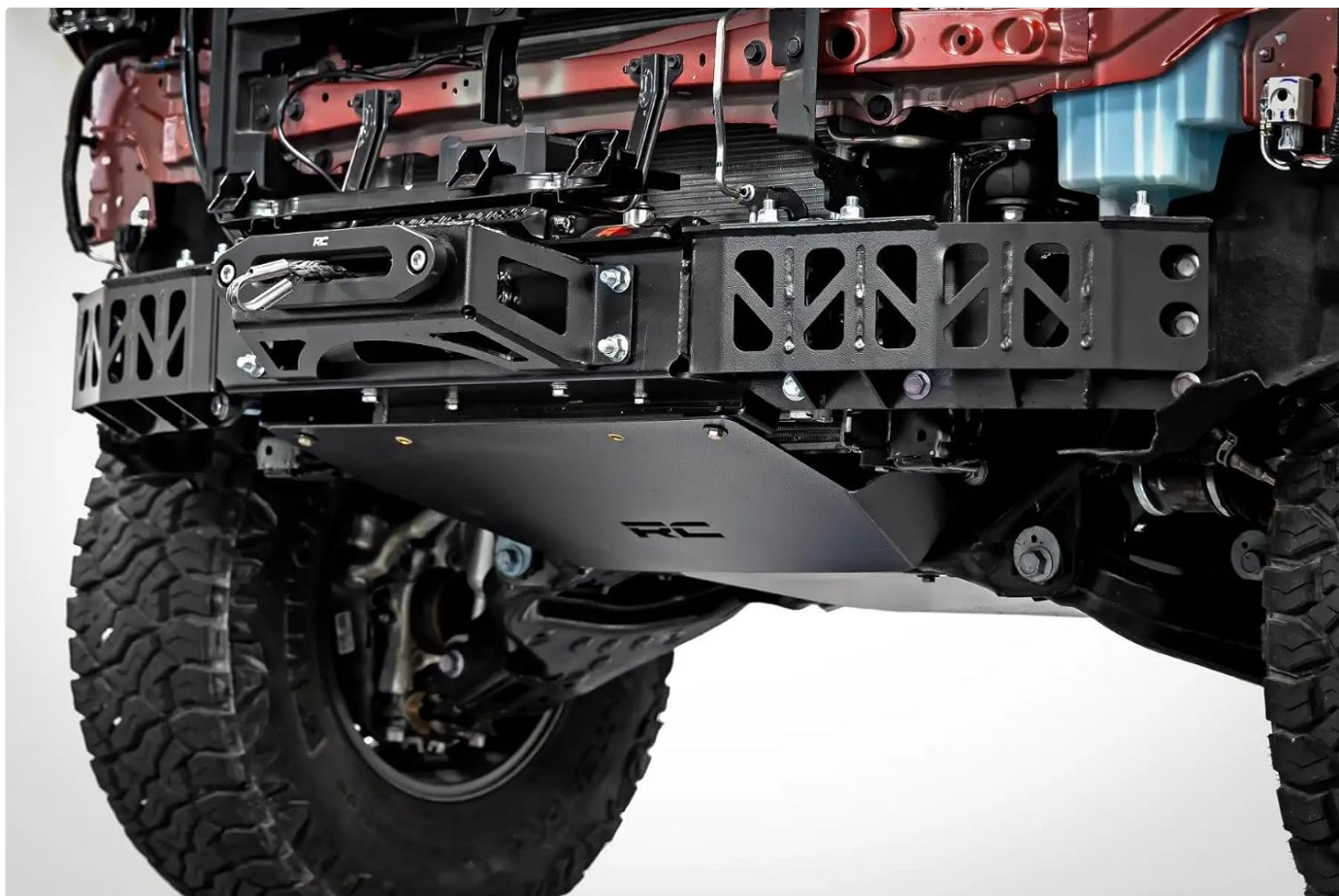
Figure 3: An alternative view of the Rough Country Hidden Winch Mount and winch installed on the vehicle chassis, showcasing the secure attachment and the differential skid plate in place.
