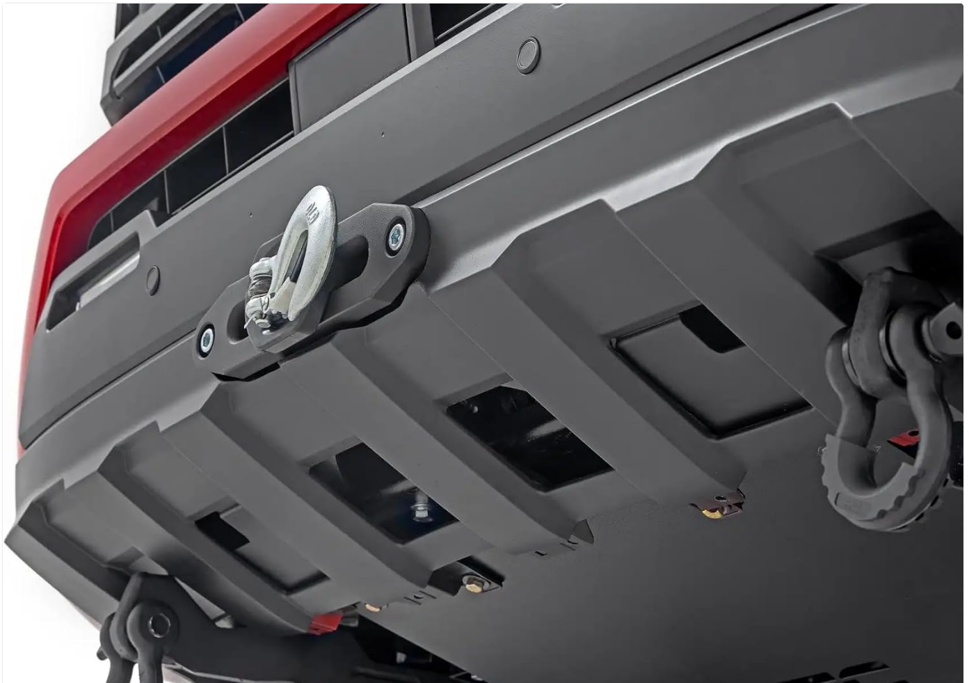
Figure 5: A close-up view of the hawse fairlead and clevis hook integrated into the front bumper, demonstrating the discreet and functional design of the hidden winch system.
