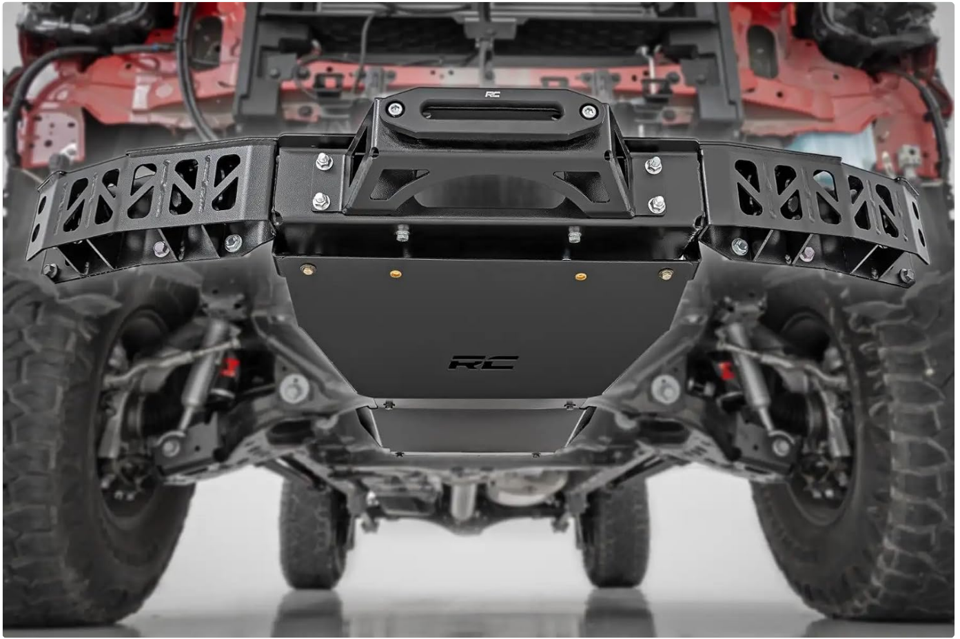
Figure 2: The Rough Country Hidden Winch Mount system and PRO12000S winch installed directly onto the Toyota Tacoma frame, prior to bumper reinstallation. This view highlights the robust steel construction and integration points.
