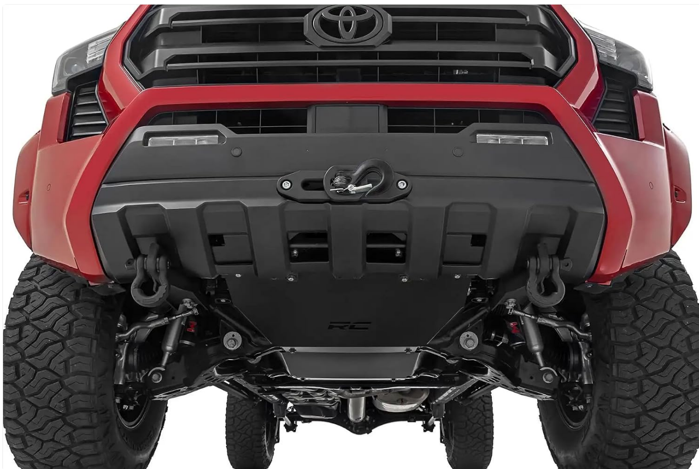
Figure 4: Undercarriage view of the installed Rough Country Hidden Winch Mount and the additional skid plate, demonstrating the
