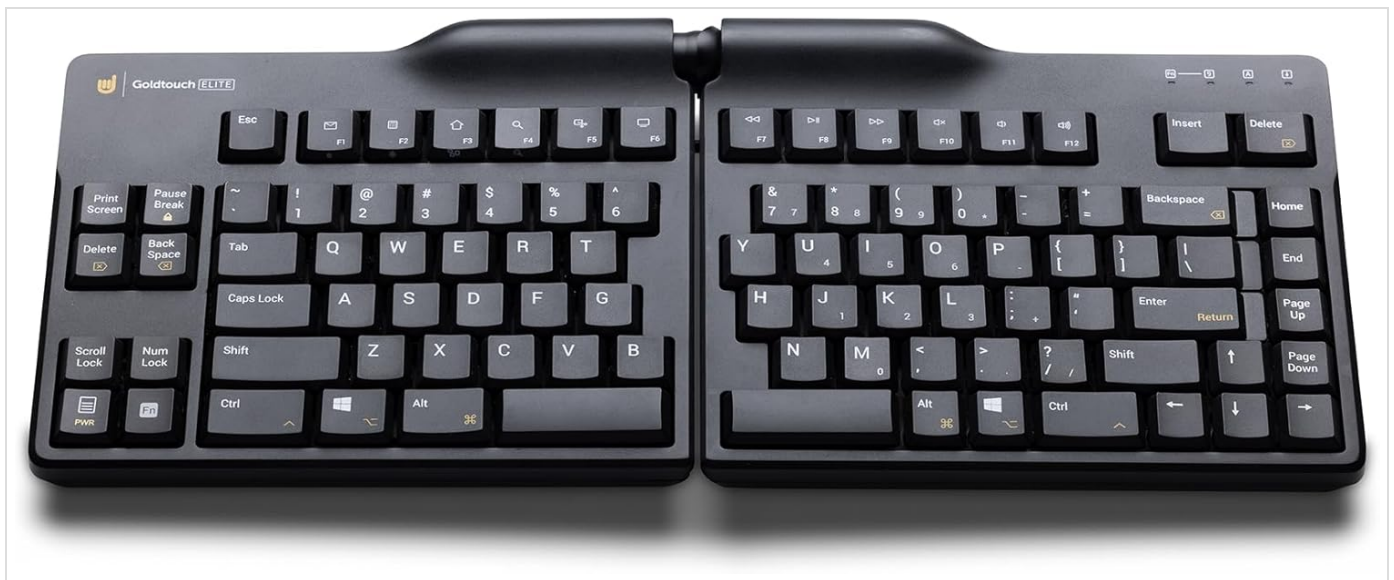
Image: The Goldtouch Elite keyboard shown in its flat, unadjusted configuration.
