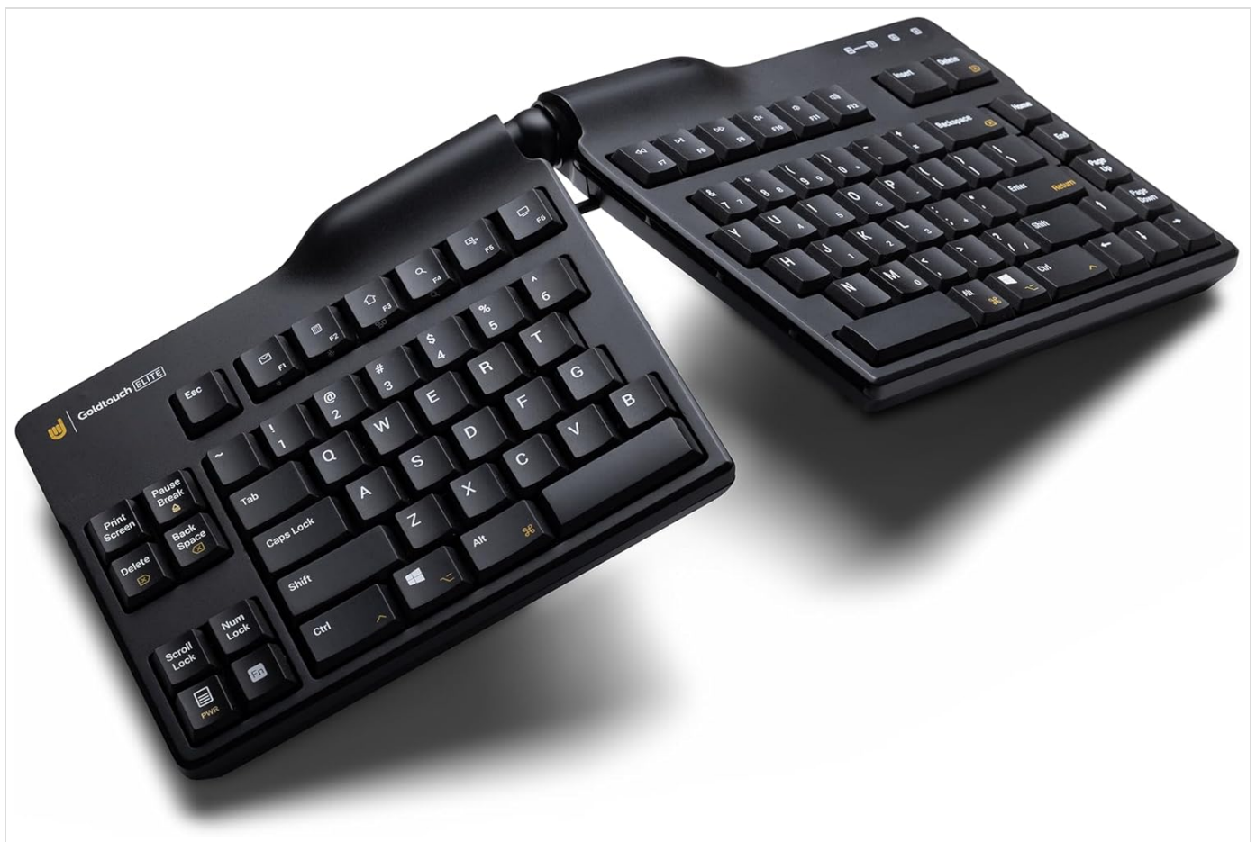
Image: The Goldtouch Elite keyboard demonstrating horizontal splay, where the two halves are angled outwards.
