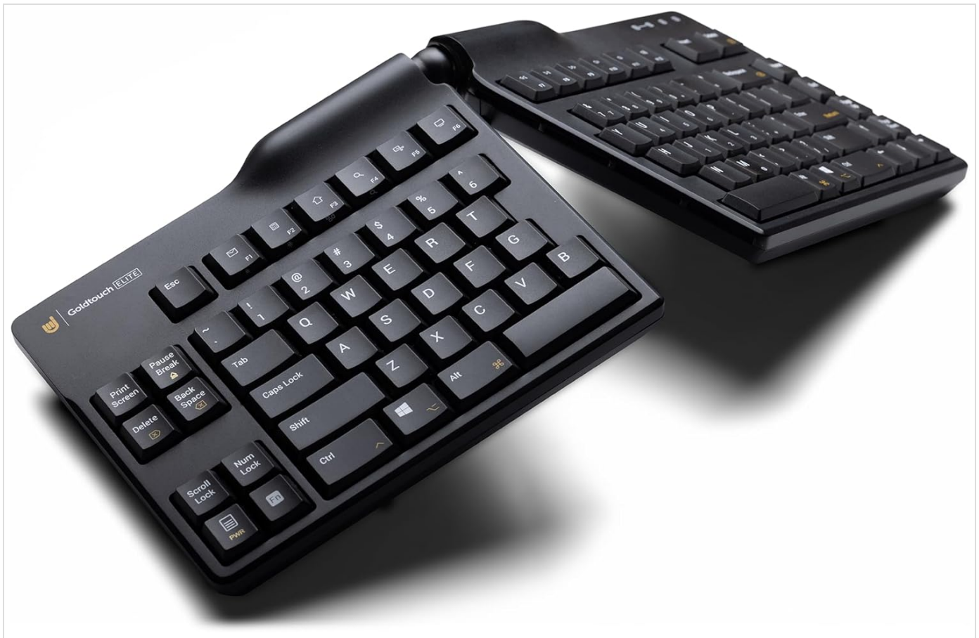
Image: The Goldtouch Elite keyboard configured with both horizontal splay and vertical tenting, elevating the inner edges.
