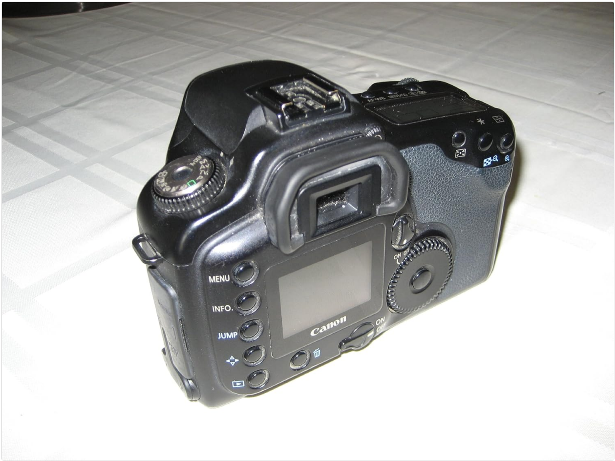
Figure 3: Rear view of the Canon EOS-10D, displaying the main LCD screen and navigation controls.
