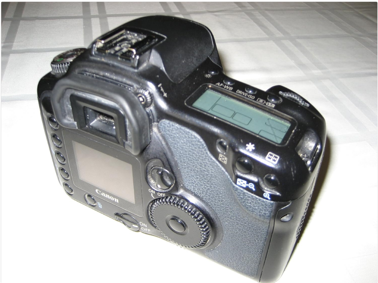
Figure 2: Top-back view of the Canon EOS-10D, highlighting the top LCD panel and various control buttons.
