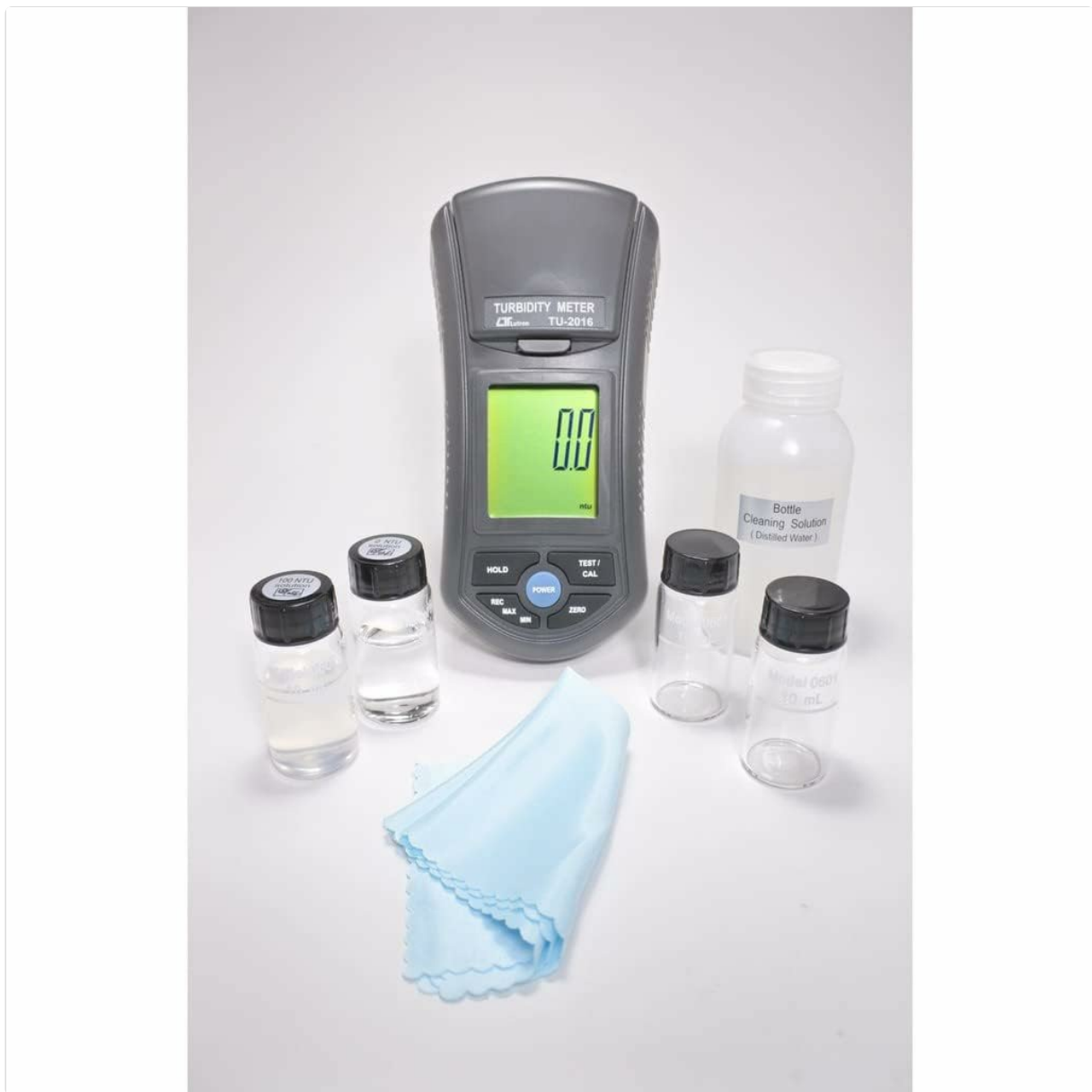
Figure 3.2: The TU-2016 Turbidity Meter along with its essential accessories for measurement and maintenance.
