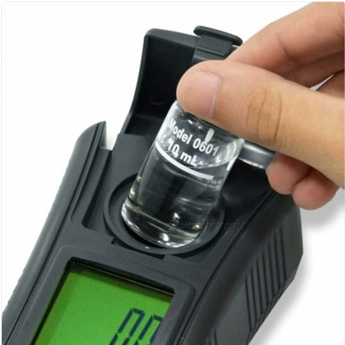
Figure 6.2: Inserting a sample bottle into the meter.
