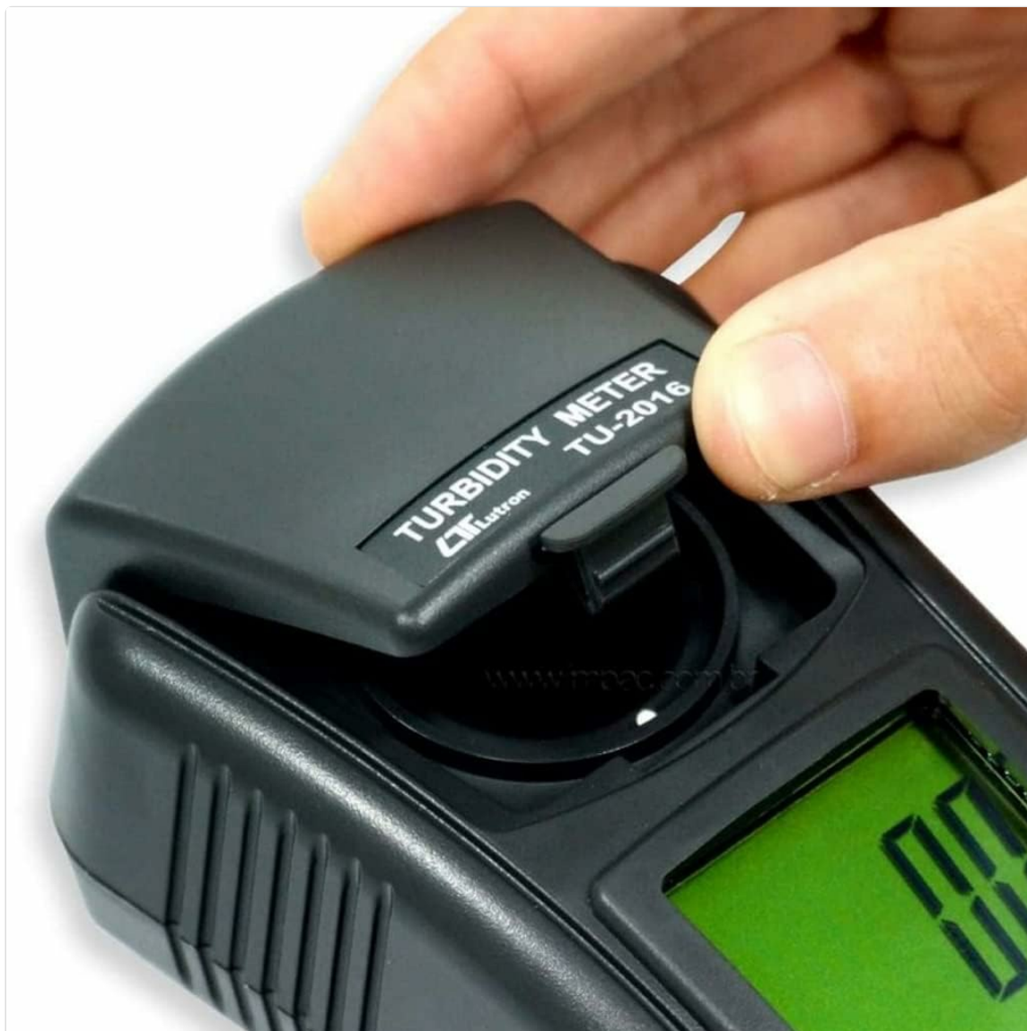
Figure 6.1: Opening the sample compartment lid.
