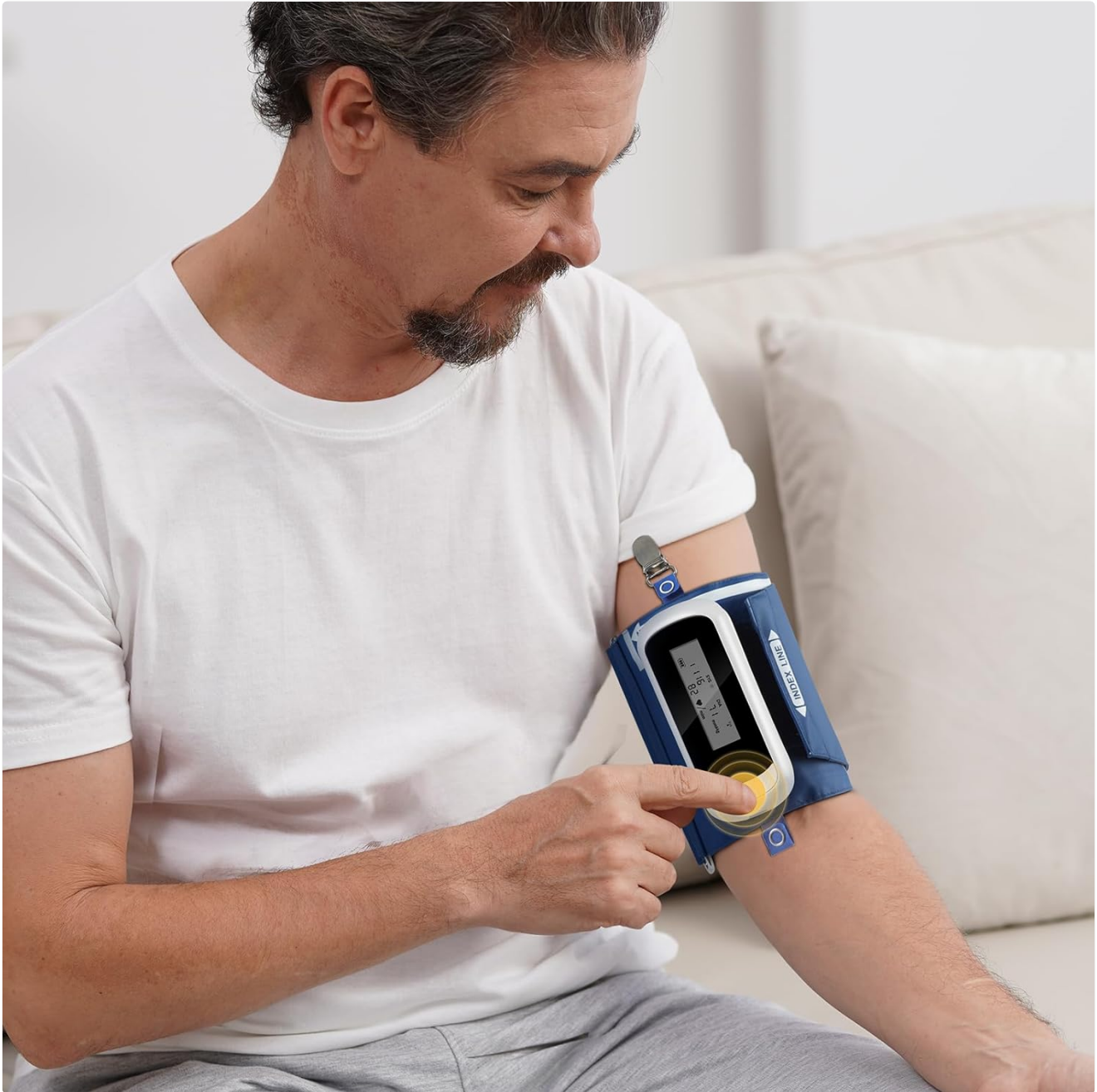
Image 4.1: Initiating a measurement on the Wellue ABPM device.
