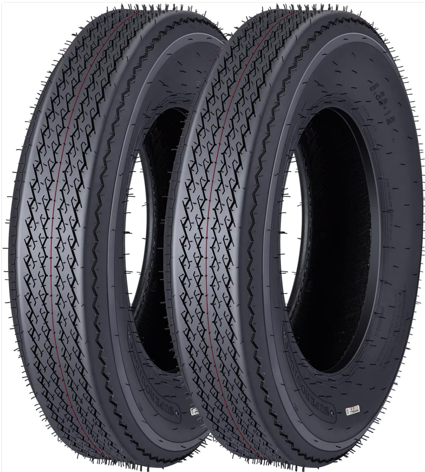
Figure 1: Two STMHOM 5.30-12 6PR Trailer Tires. These tires feature a robust construction suitable for trailer use.
