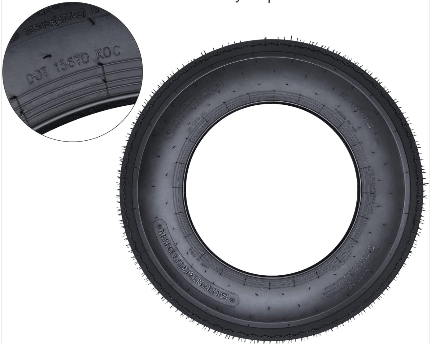
Figure 2: Tire Sidewall Information. Each tire has its size and load specifications branded on the sidewall. Always verify this information before installation.
