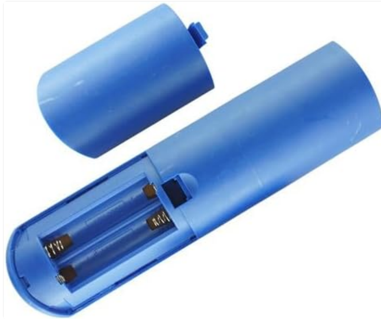
Image 2.1: View of the remote control's battery compartment, showing the correct orientation for AAA battery insertion.
