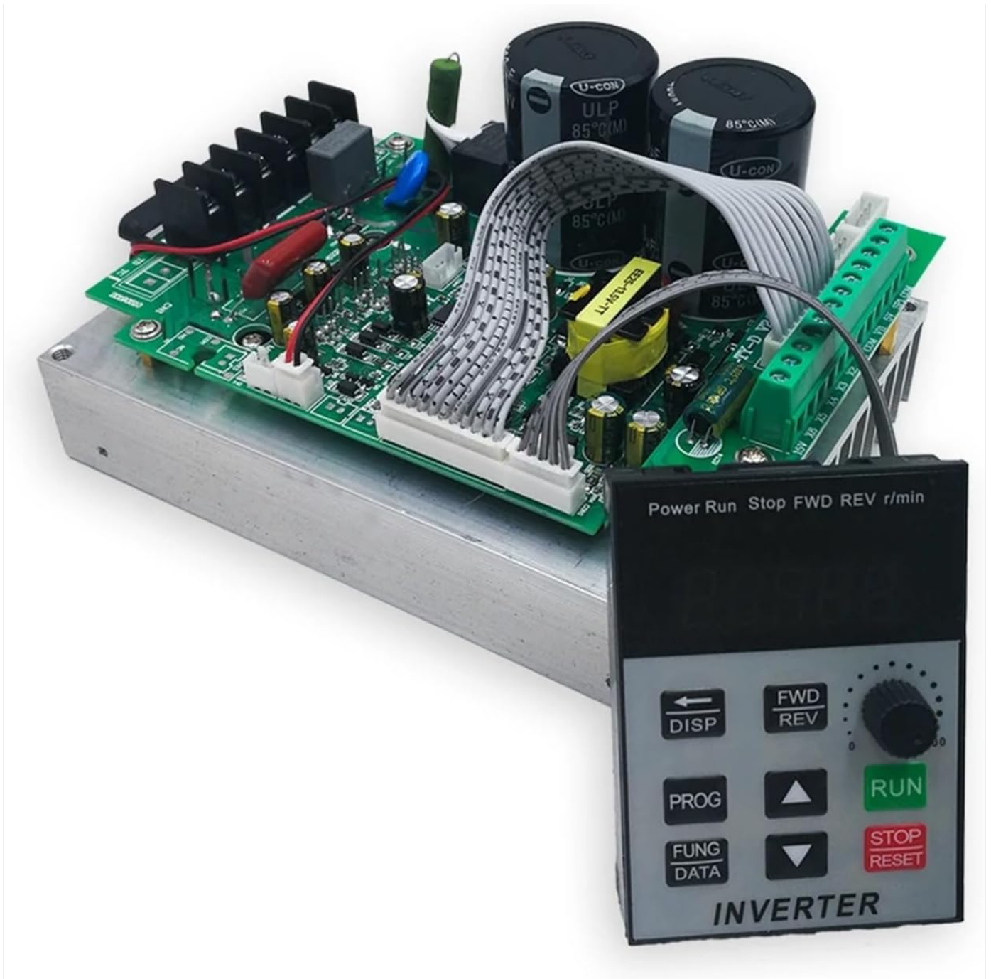
Image 6.1: View of the internal components of the XSY-AT1 VFD, demonstrating its construction, alongside the remote control panel.
