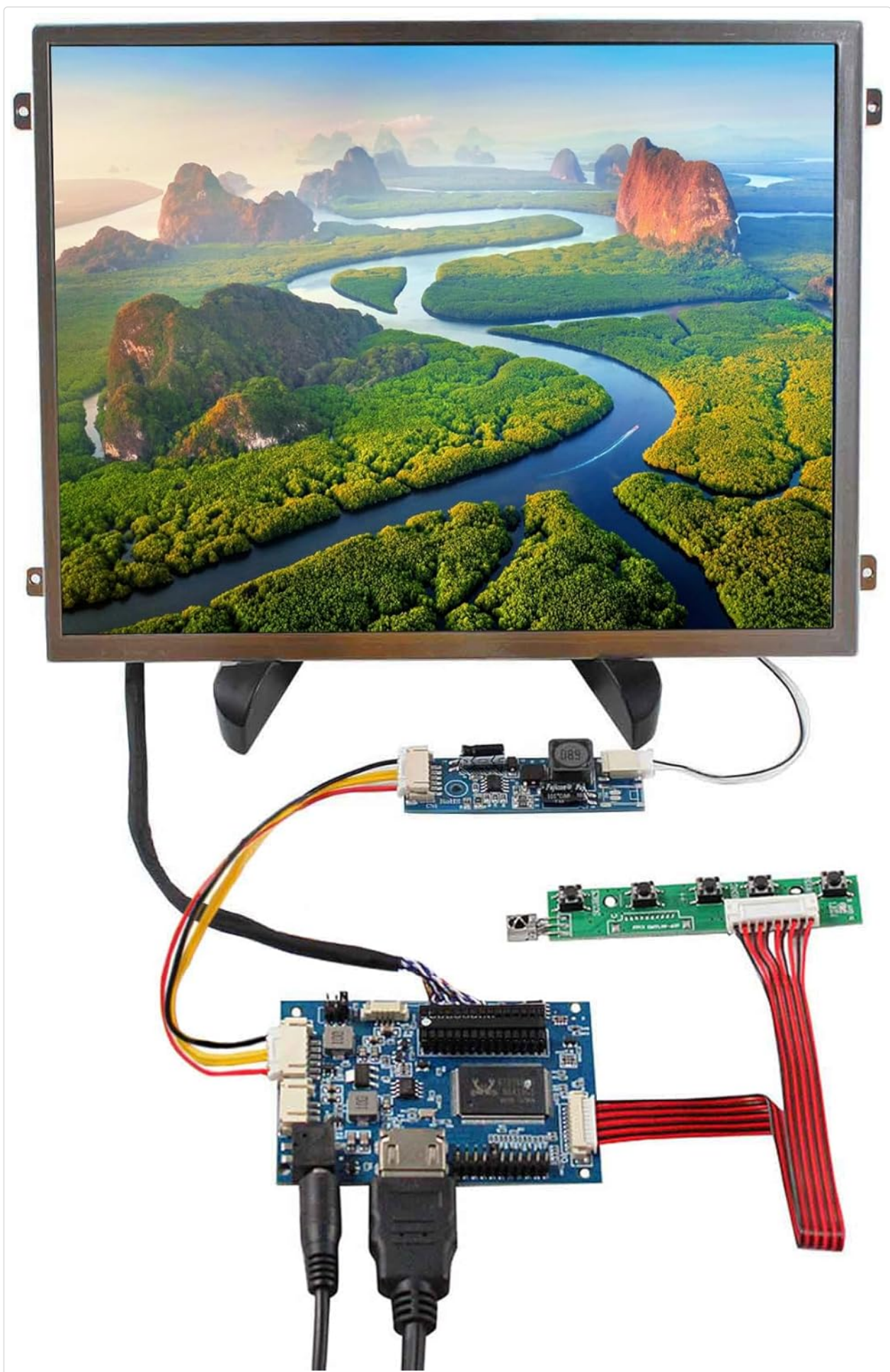
Figure 5.1: Fully assembled VSDISPLAY LCD screen and controller board setup.
