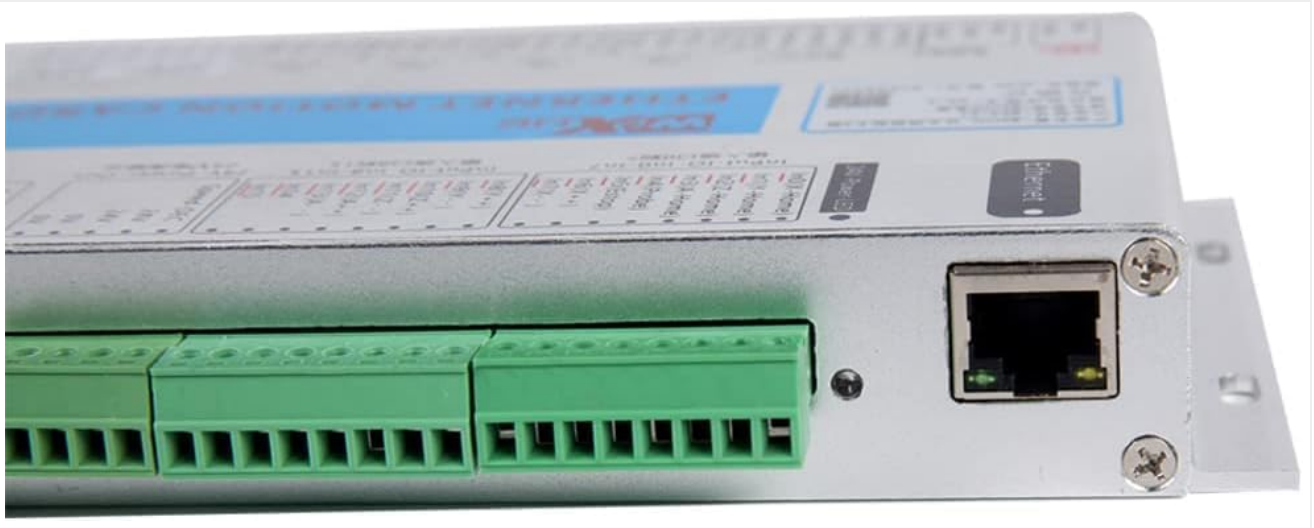
Figure 4.3.1: Close-up view of the WiXHC MK4-V Motion Control Card showing the USB port, Ethernet port, and various terminal blocks for input/output connections. The board is silver with green terminal blocks.
