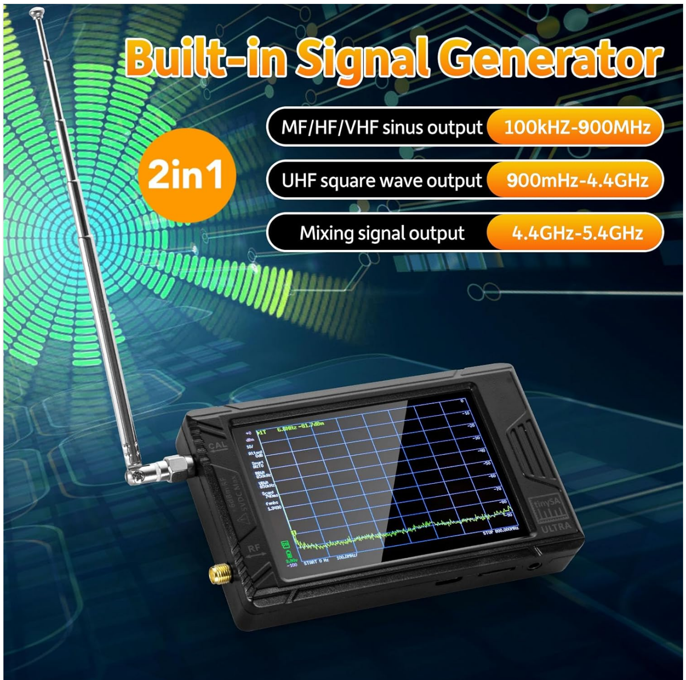
Image 5.1: The TinySA Ultra+ displaying its signal generator capabilities, including MF/HF/VHF sinus, UHF square wave, and mixing signal outputs.
