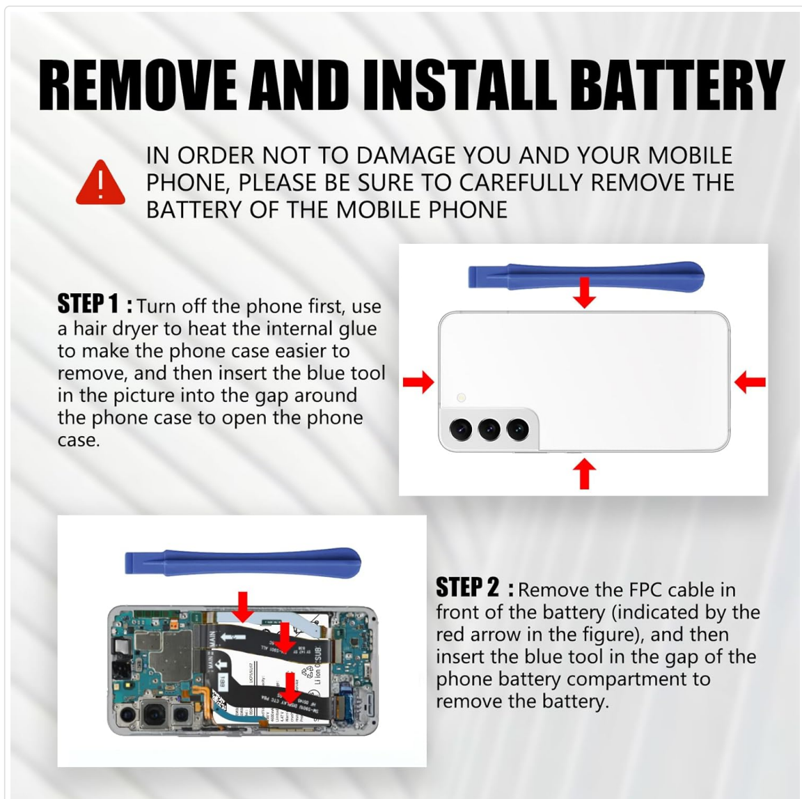
Image 4.1: Illustration of carefully opening the phone's back cover using a prying tool after heating the adhesive.
