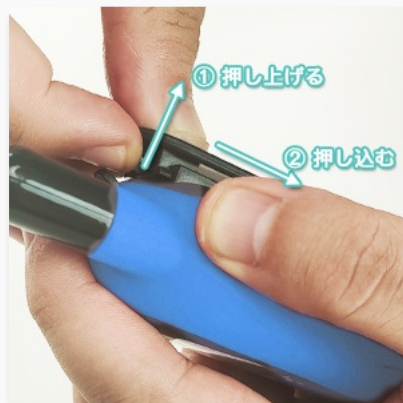
Figure 4: Steps for attaching the belt clip to the transceiver.
