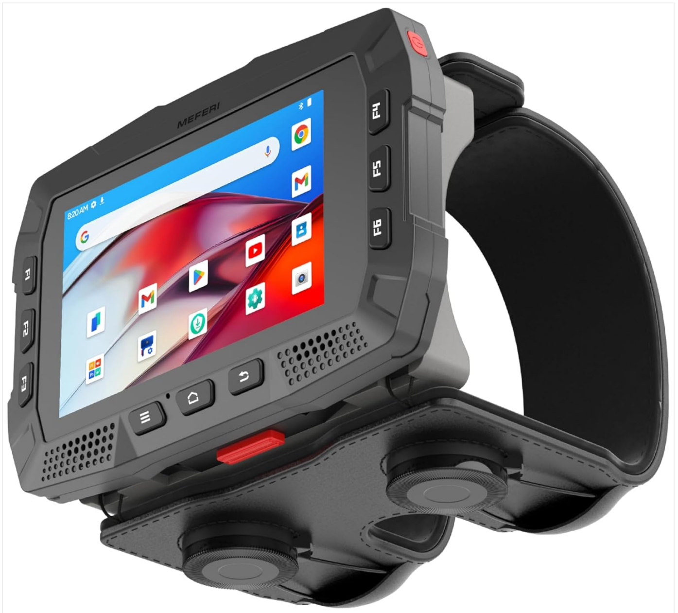
Figure 1: MEFERI ME10 Wearable Computer mounted on a wrist strap, displaying its user interface.
