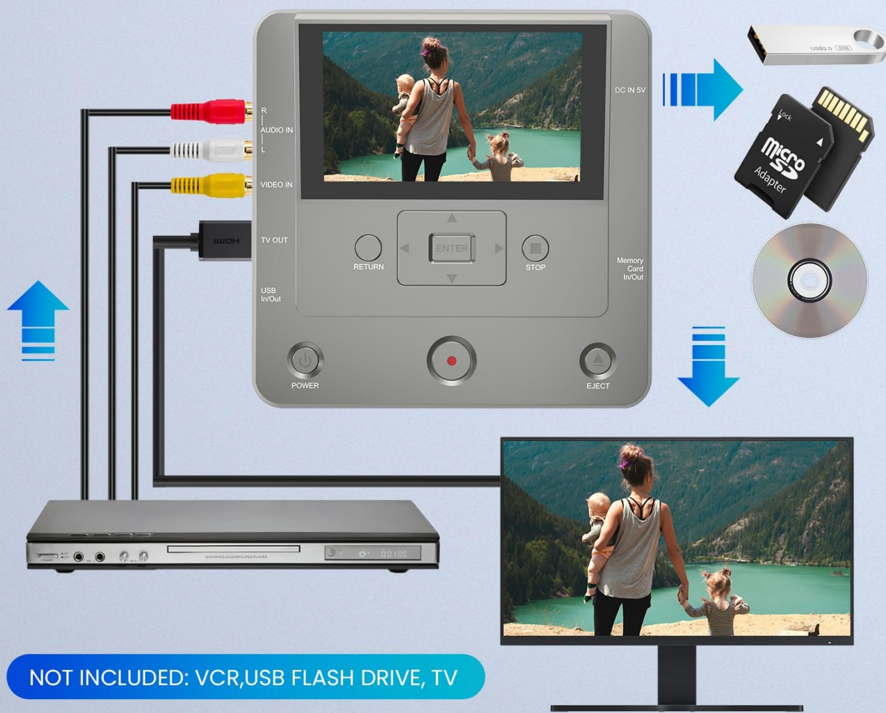
Image: A visual guide illustrating how to connect a source device (like a DVD player) to the KOHO KR043B using RCA cables for video and audio input, and how the recorder can output to a TV or store to USB/SD/DVD.
