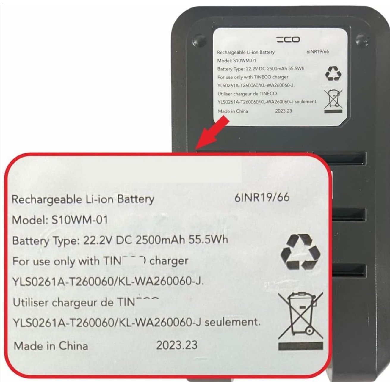
Image 8.1: Detailed view of the battery label, confirming model, voltage, capacity, and compatible charger information.
