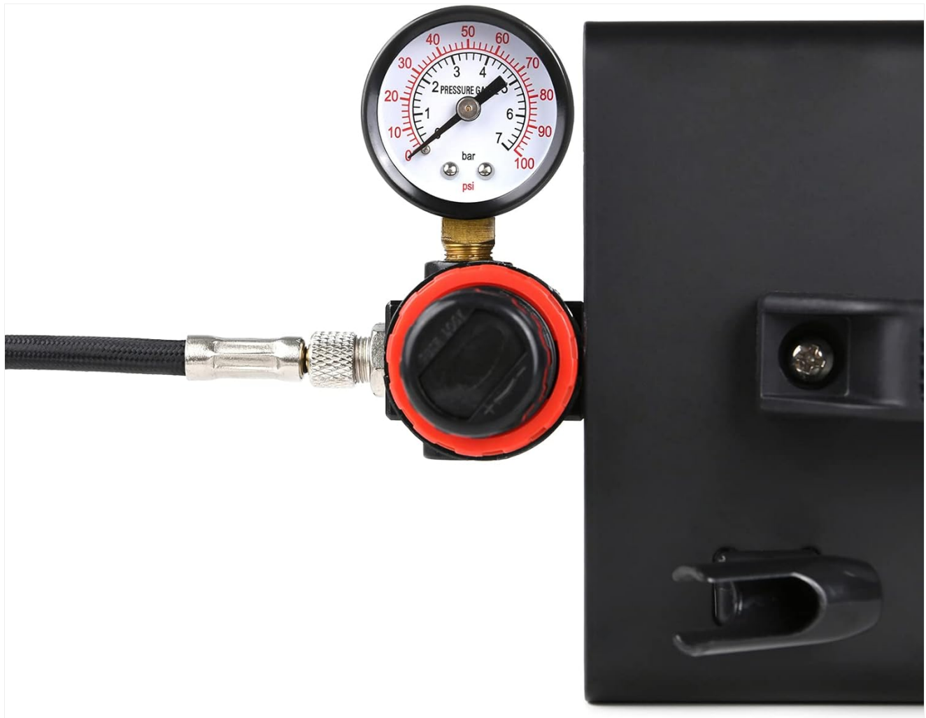
Image 3.1: A close-up view of the air pressure gauge and regulator on the compressor. This component allows for precise control over the air pressure during operation.
