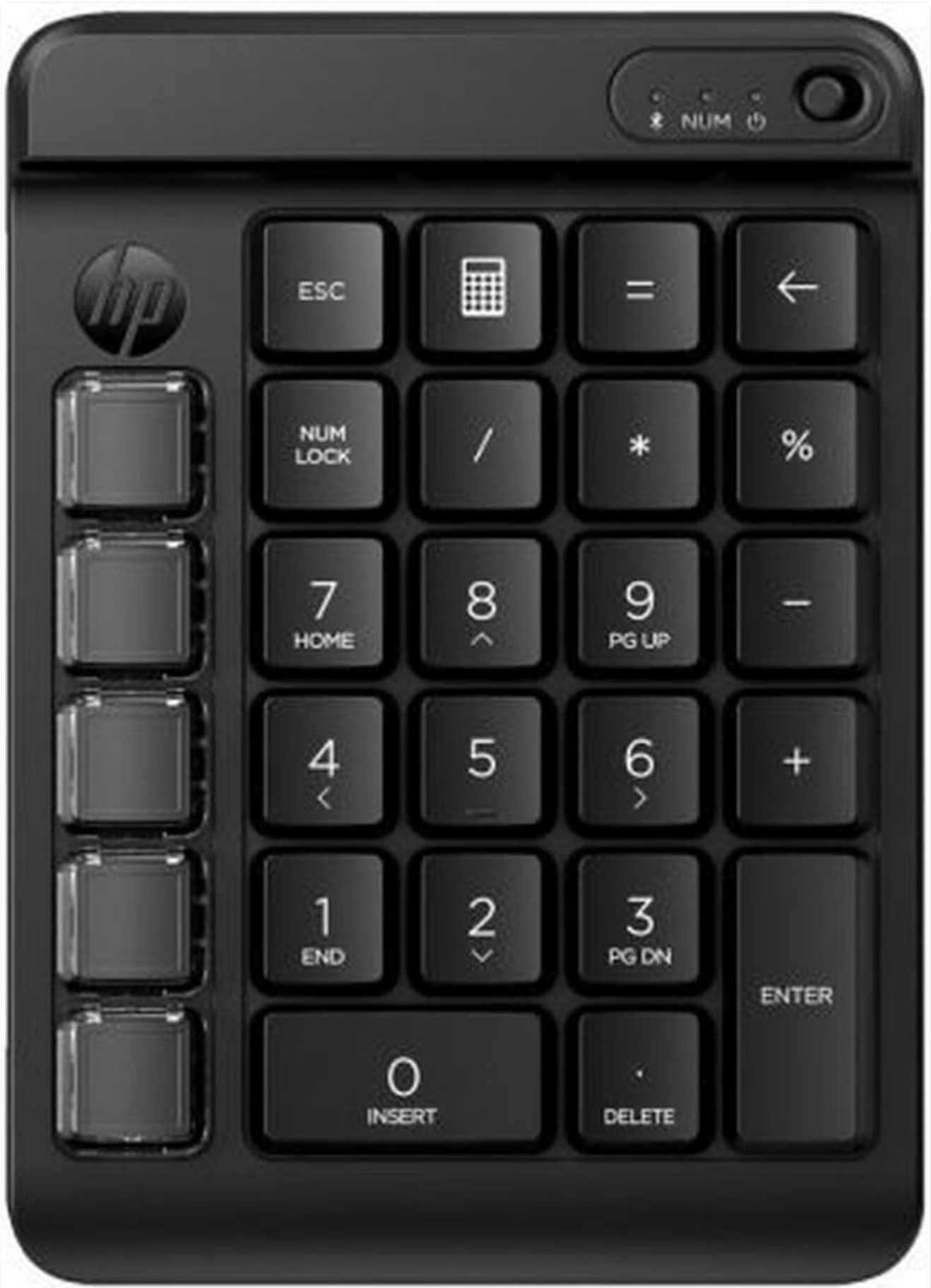
Figure 1: HP 435 Programmable Keypad, front view. This image displays the black keypad with its 9 customizable keys on the left side and the standard numeric keypad layout on the right. Key labels such as ESC, NUM LOCK, ENTER, and DELETE are visible, along with a power button and NUM Lock indicator light at the top.
