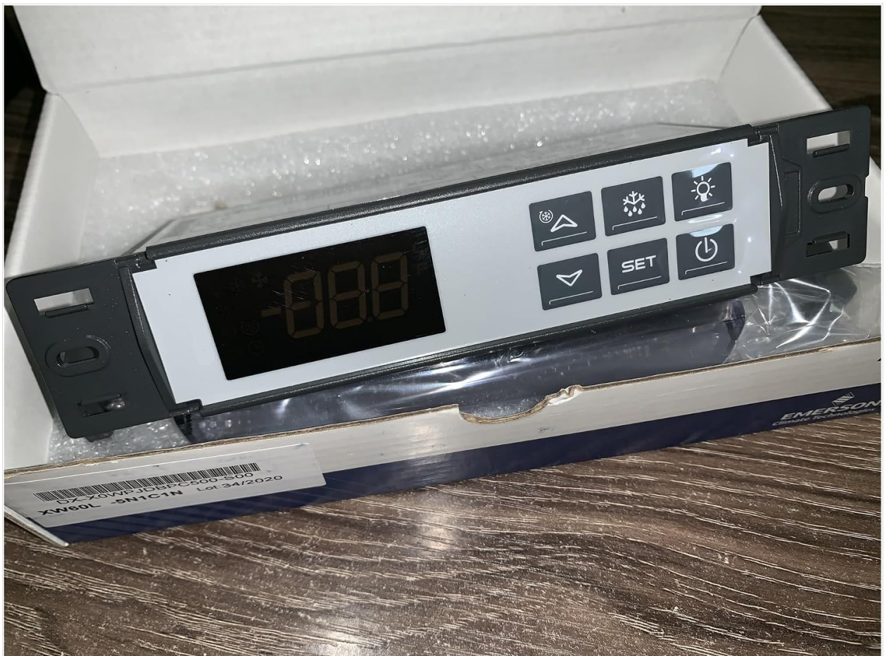
Figure 3.2: Close-up of the controller's front panel, featuring the digital display and control buttons. The buttons include 'Up', 'Down', 'SET', 'Power', 'Defrost/Snowflake', and 'Light/Fan', providing direct interaction for setting parameters and controlling functions.
