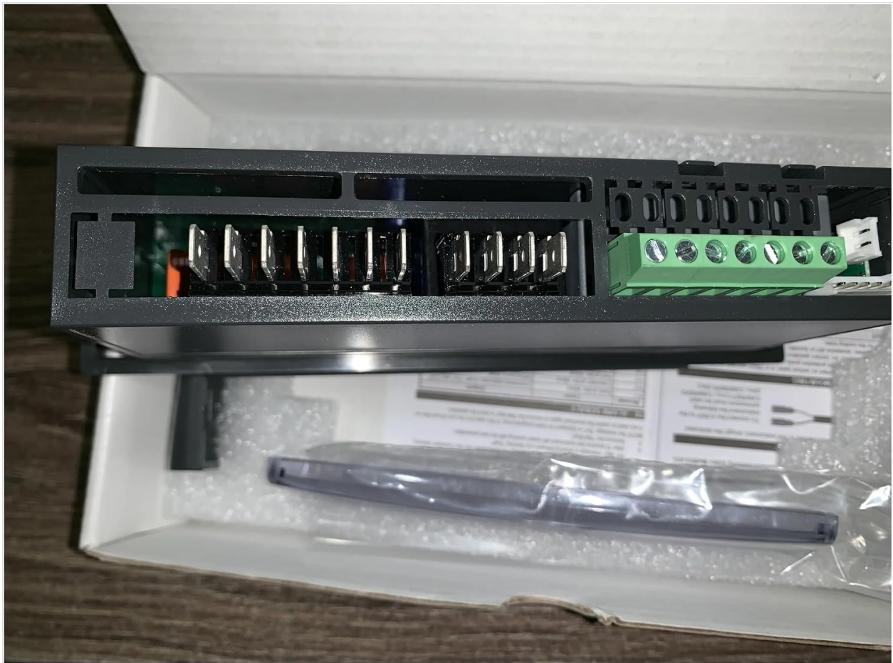
Figure 3.3: Side view of the Aoleaby XW60L-5N1C1-N controller, illustrating the terminal blocks for electrical connections. This view provides a clear perspective on the physical interface for wiring the device into a system.
