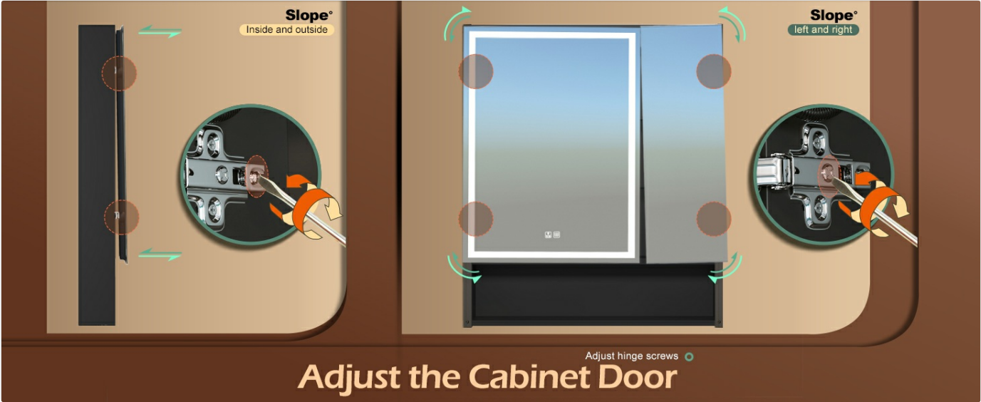
Figure 4.2.1: Adjusting Cabinet Door Hinges
