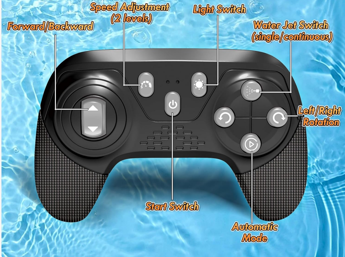
Image: A detailed diagram of the 2.4GHz remote control, labeling buttons for forward/backward movement, speed adjustment (2 levels), light switch, water jet switch (single/continuous), left/right rotation, start switch, and automatic mode.
