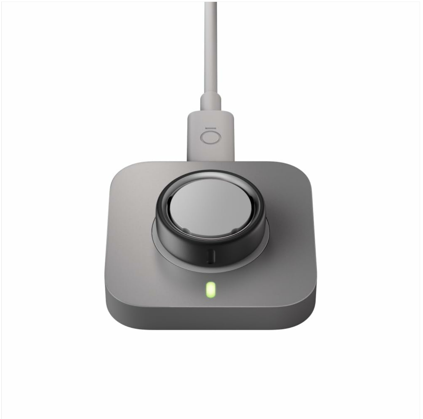
Image: An OURA Ring 4 placed on the charging dock, with a green indicator light showing that it is actively charging.
