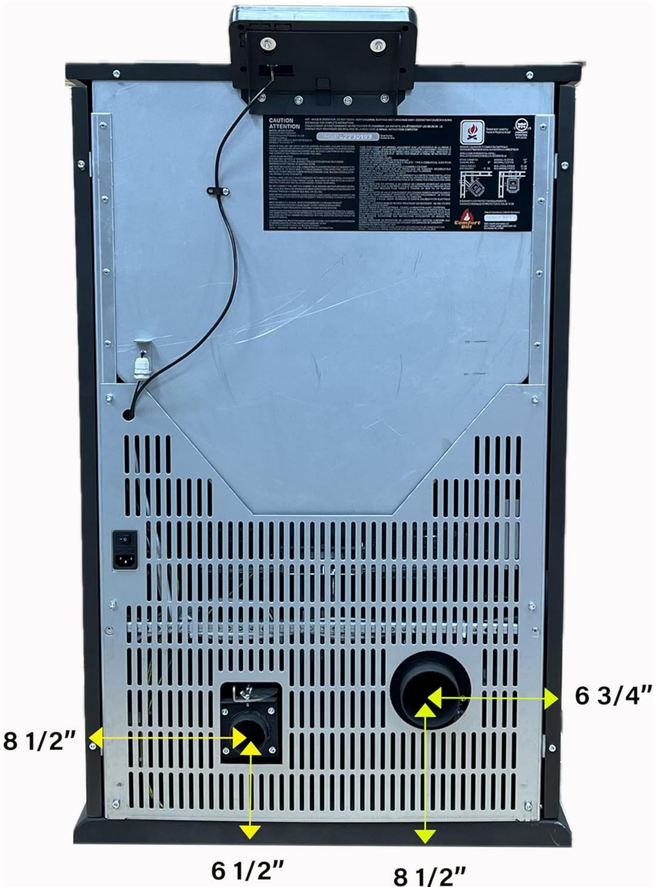
Image: Rear view of the Comfortbilt HP42-Alpine pellet stove, highlighting the exhaust and air intake connections. Key dimensions for these connections are shown: 6 3/4 inches from the bottom to the center of the exhaust, 6 1/2 inches between the centers of the exhaust and air intake, and 8 1/2 inches from the sides to the centers of the connections. This is vital for proper venting installation.
