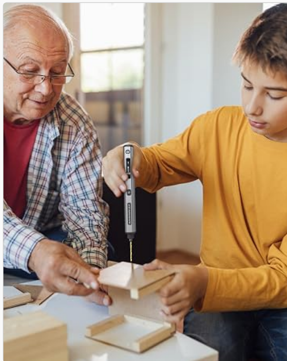
Image 5.1: An individual demonstrating the use of a rotary tool with an ARROWMAX carving bit for intricate detailing on a small workpiece.
