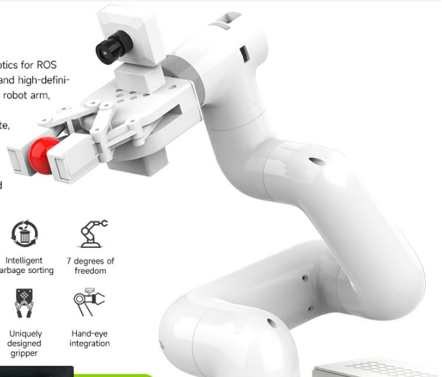
Image 1.1: Overview of the Yahboom Jetcobot Robotic Arm, highlighting its collaborative design and integration with Jetson Orin Nano.
