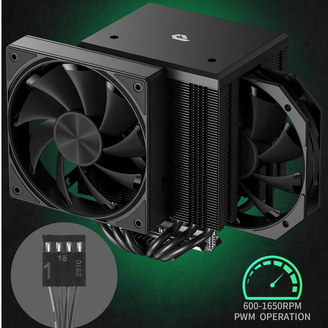
Image 4.3: The dual tower design and PWM fan control contribute to efficient cooling.
